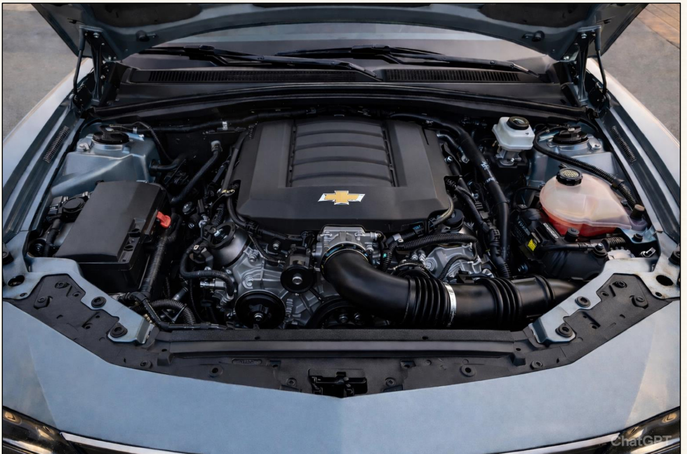
LT1 6.2L OHV V8 push rod design, aluminum block, 450 HP naturally aspirated, 400 lb-ft torque
