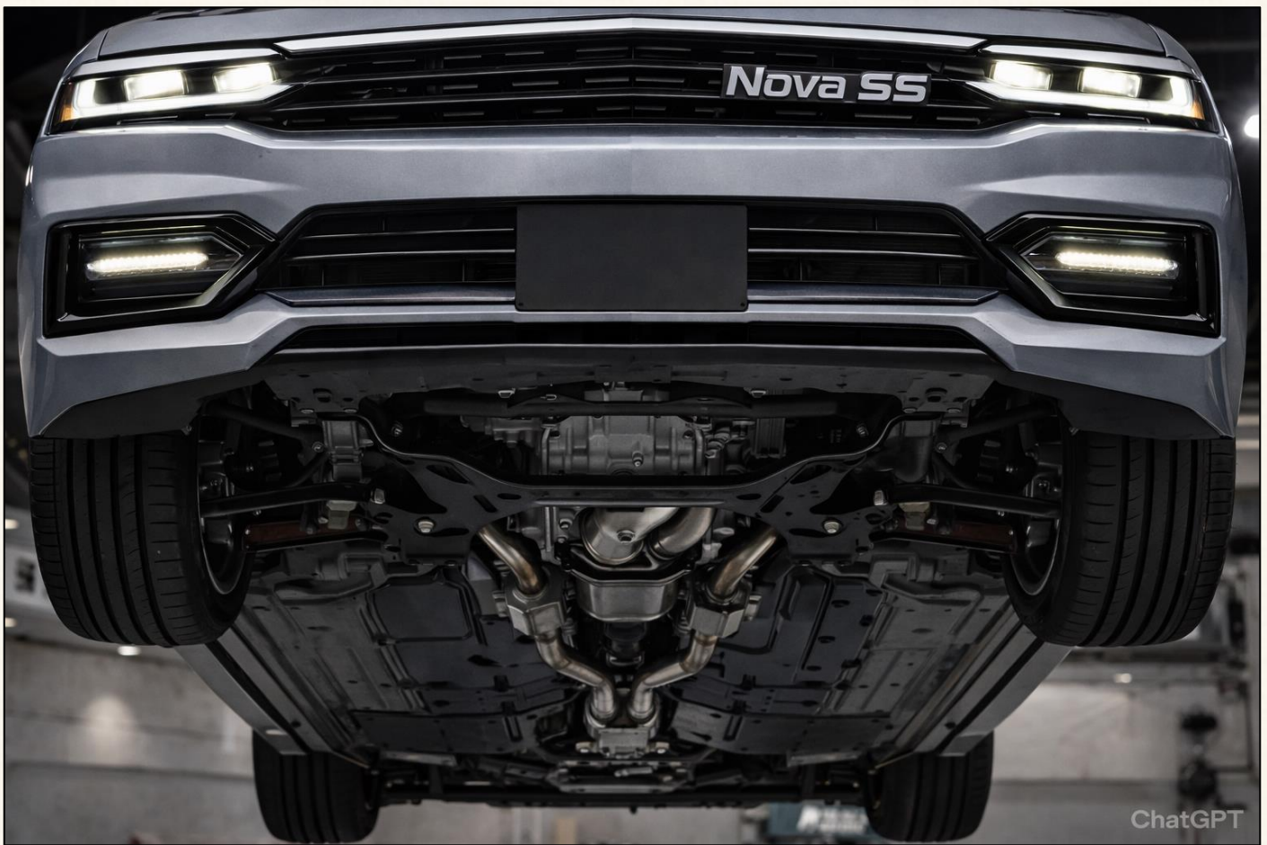
Double wishbone, aluminum components, coilovers, large sway bar
