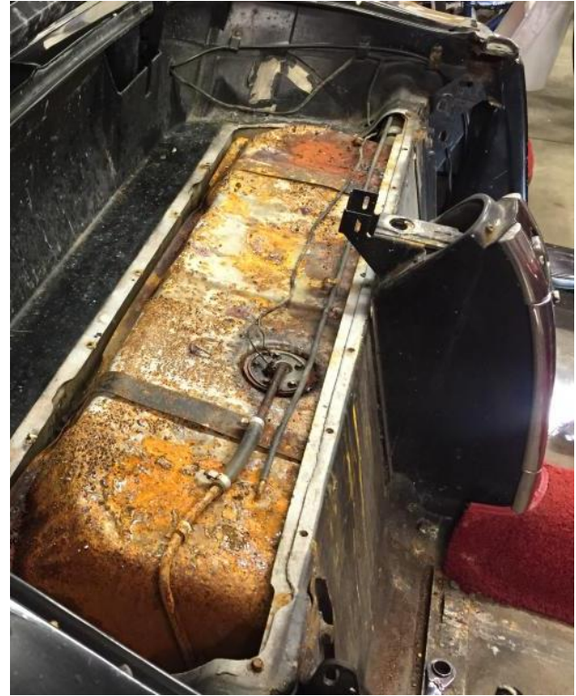
Rusted C1 Gas Tank
