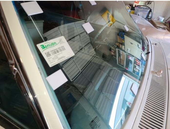
New glass was installed
