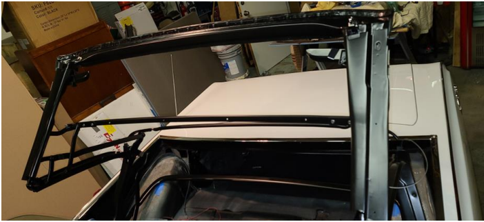
Convertible roof frame now like new
