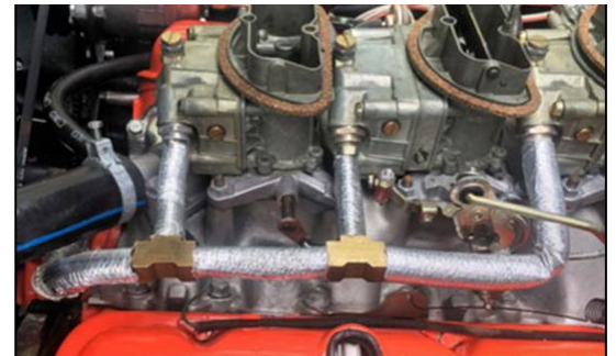
Insulation added to Corvette Tri-Power carburetors
