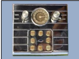
1938 Master Deluxe, push button control head, AC Spark Plug
