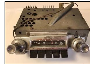
1962 Impala all transistor AM, push button, Delco 985264
