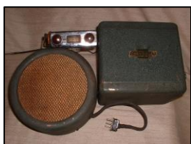
Firewall mounted radio, interior control head & enclosed speaker box
