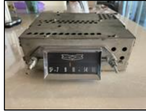
1957 Chevy AM, vacuum tube transistor hybrid, Delco 987573
