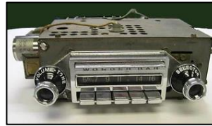
1958 Wonder Bar AM push button radio, transistor hybrid, Delco 987730
